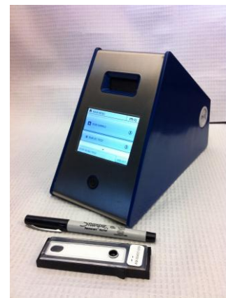
Figure 1. MBio multiplexed immunoassay system, including a reader and disposable cartridges.
