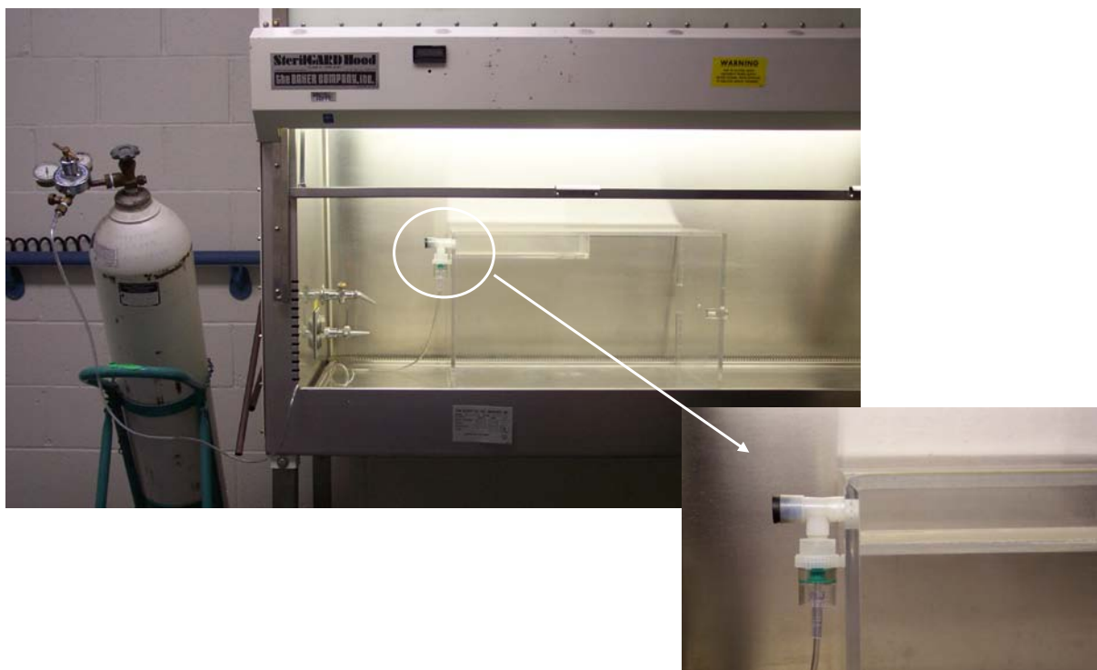
Figure 2. Madison Inhalation Chamber Apparatus for Aspergillosis
