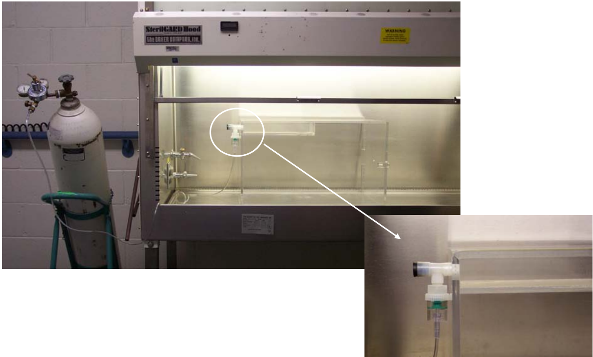
Figure 1. Acrylic Inhalation Chamber Apparatus for Aspergillosis
