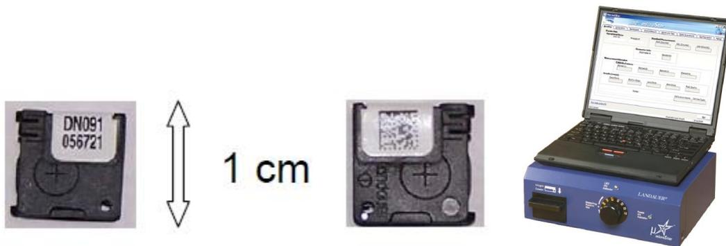
**Figure 11.** Nanodot OSLD dosimeter and reader.
