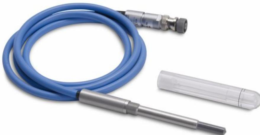
**Figure 4.** Farmer type ion chamber
